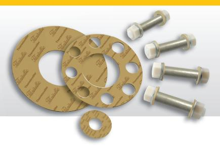
The insulating gasket is constructed from a serrated metal core with unique profile. The metal core is faced with Thermiculite® 725; a high performance, fire safe sealing material incorporating Flexitallic's proprietary vermiculite based sealing material. Correct gasket location is ensured by the inclusion of a Thermiculite® 725 spacer ring positioned around the periphery of the serrated metal core.
